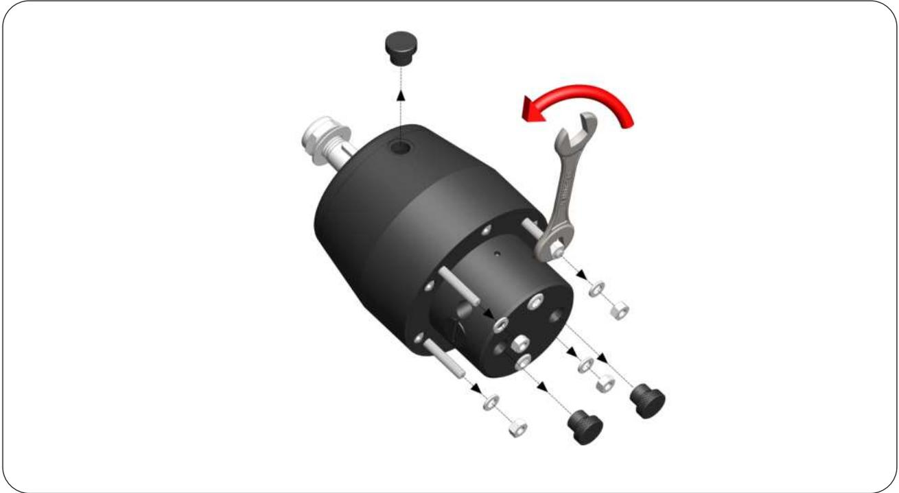
**STEP 5 :** Insert and tighten by hand the Elbow Fittings (1) until they are fully seated, then tighten with a wrench. Turning again from 1.5 to 2.5 turns, for their best orientation for the Hose connection. However do not exceed a maximum torque of 17.6 Nm (13 lb ft). Also insert the Oil Filling Plug with Breather Hole (2) into Oil Filling Port
