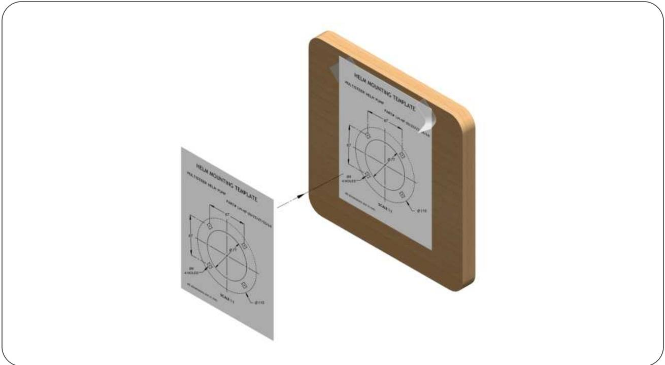
**STEP 3 :** Make 4 holes for the flange studs with the help of a Hand Drill and a big one for the center hole with the help of hole saw.
