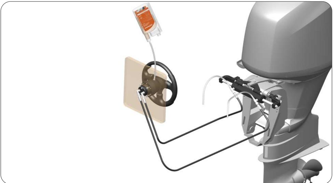
**STEP 13 :** Turn the Steering Wheel slowly towards Starboard Side, so that the Oil can come out of Hoses. Unscrew the Port Side air bleeder and allow the air & Oil (air bubbles) come out from air bleeder.
