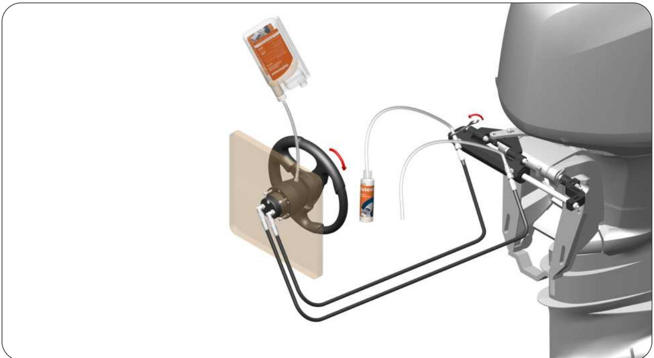
**STEP 17 :** After completion of purging process, remove the Oil Bottle, Oil Filling Kit & Oil Collection Kit. Insert the Oil Filling Plug and Protective Caps.
