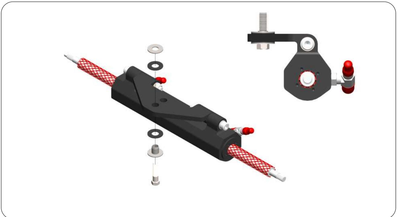
**STEP 5:** Position the Engine straight so that its Engine Arm is perpendicular to the Transom. Connect the Tiller Arm (2) of Cylinder to the Engine Arm by means of the Hex Stud (5). Tighten it by using a 14mm Wrench with a torque of 20 Nm (14.75 lb ft). Tighten the Nyloc Nut of Hex Stud by using a 14mm Wrench with a torque of 20 Nm (14.75 lb ft). After tightening the Nyloc Nut, check for the right torque 20 Nm (14.75 lb ft) of the Hex Stud (5).
