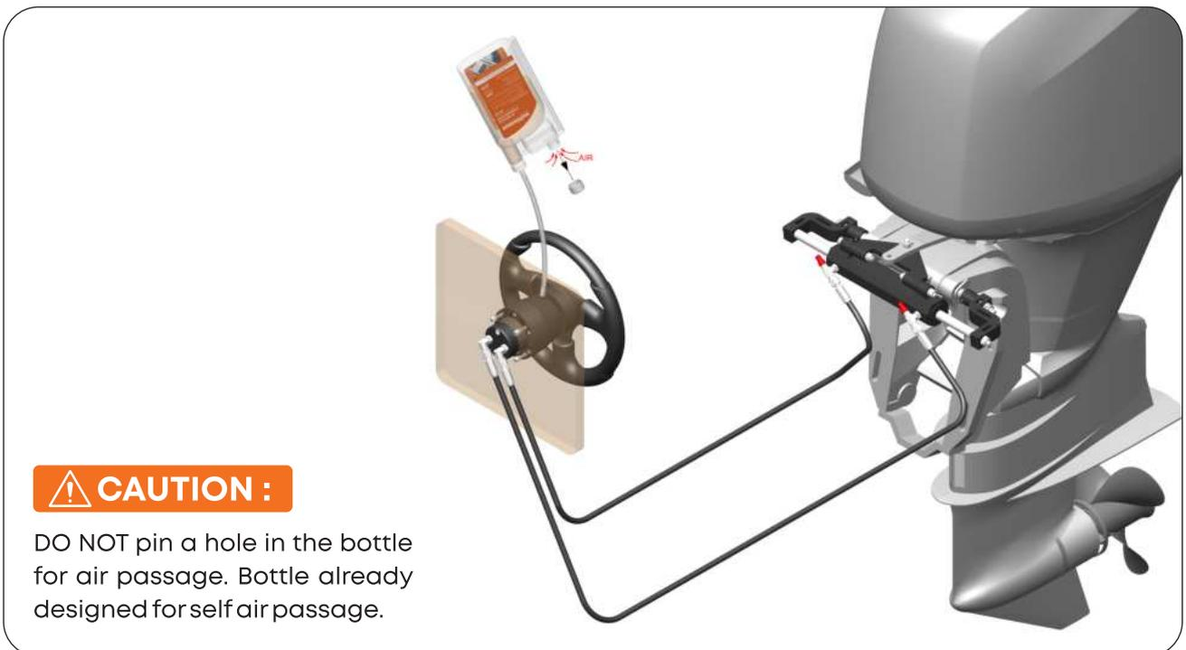
**STEP 11:** Remove the Protector Cap of both the air bleeders.
