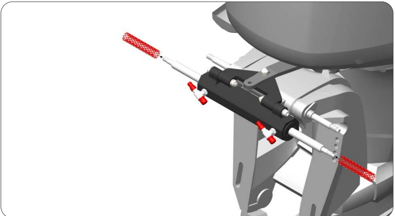
**STEP 7:** Insert the Mounting Spacer (8), Delrin Spacer Big (6), Delrin Washer Small (7) & Washer (10) as show. With reference to the "Application Guide" Choose the correct number of washers for the tilt tube rod. In this phase ensure that the Cylinder body is centered on the Piston Rod (1) and that the Engine is perpendicular to the Transom.
