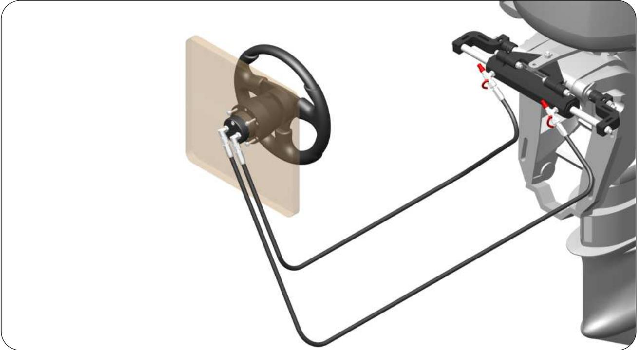
**STEP 6 :** Ensure that all the Hose Fittings should be tighten properly. Hoses should not be bent in excess. Minimum Hose bent radius is 100 mm (4 Inch). Ensure that there should be no interference during engine tilting as well as no interference with the transom.
