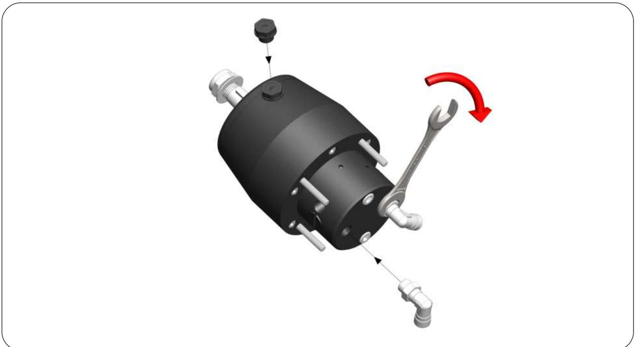
**STEP 6 :** Insert the Helm from the front of the dashboard with the Oil Filling Plug (2) turned upwards matching the 4 Flange Studs (5) moving inside the 4 holes on the dashboard.
