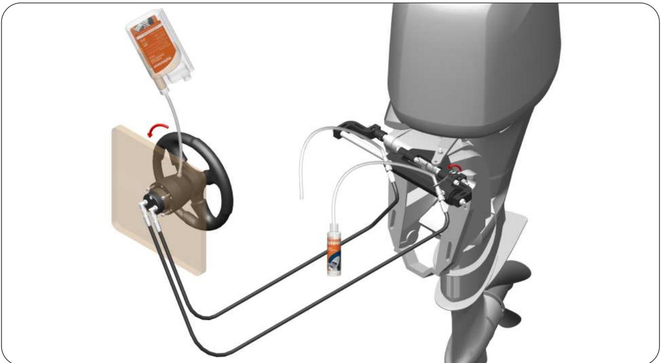
**STEP 15 :** Similarly turn the Steering Wheel slowly towards Port Side, so that the Oil can come out of Hoses. Unscrew the Starboard Side air bleeder and allow the air & Oil (air bubbles) come out from air bleeder.
