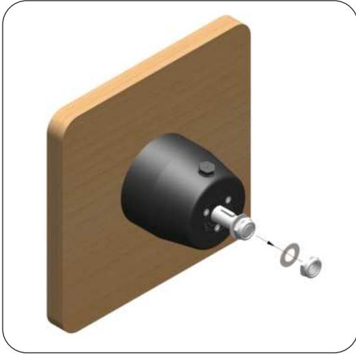
**STEP 1:** Remove the Nylock Nut (6) & Washer (8) from the Helm Shaft.
