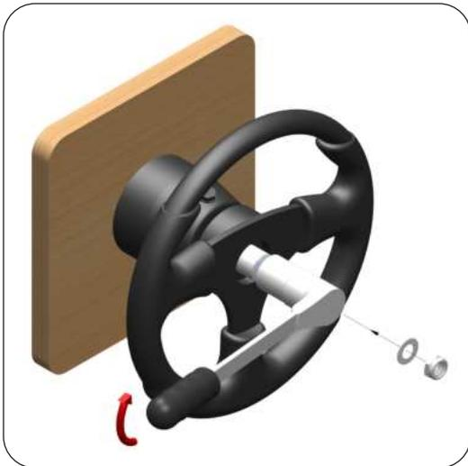
**STEP 3 :** Fit the Steering Wheel on the Shaft by inserting the Specific Key (4) in its compartment. Insert the Washer (8) and use a 20mm Hexagonal Wrench to tighten the Self-Locking Nut (6) with a 40 Nm (29.5 lb ft) torque.
