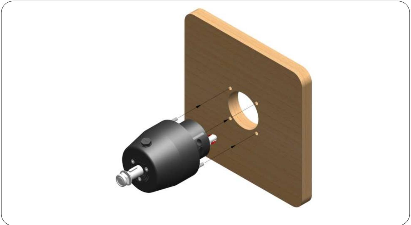
**STEP 7 :** Tighten the 4 Hex Nuts (7) & the 4 Washers (9) through the Flange Studs (5) of the Helm to the dashboard with the help of a 10mm Wrench with the torque of a 10 Nm (7.4 lb ft).
