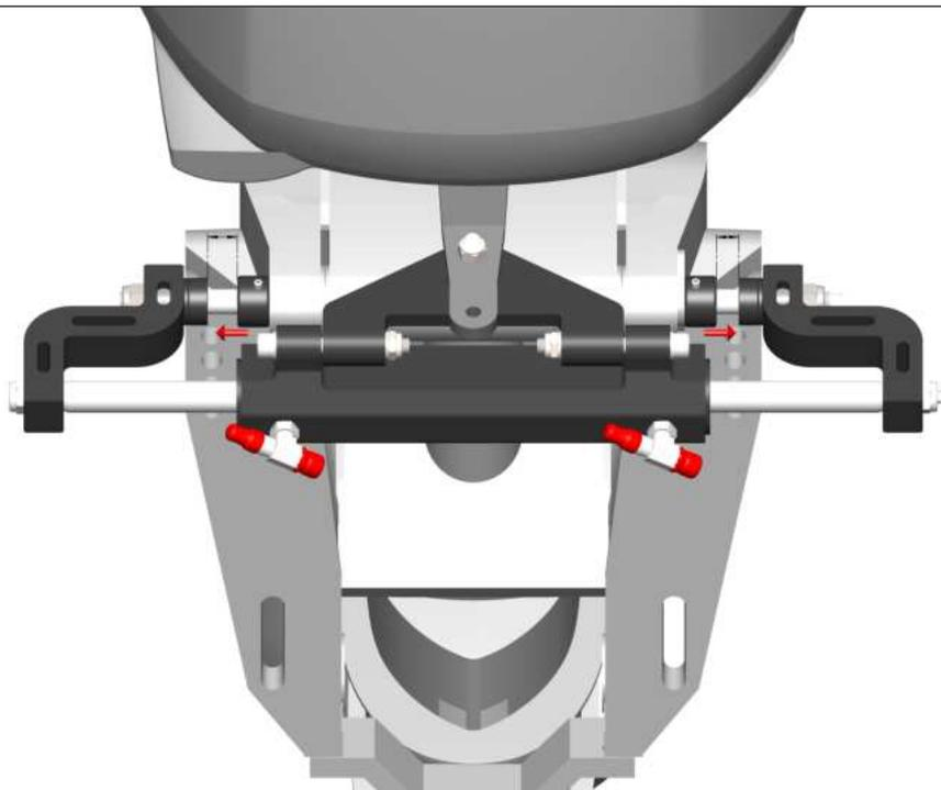
**STEP 11:** Verify if the Cylinder installation is correct by manually moving the engine on the Starboard & Port side. The displacement must be as symmetric as much as possible between Port and Starboard so that the Steering angle is the same on both sides.
