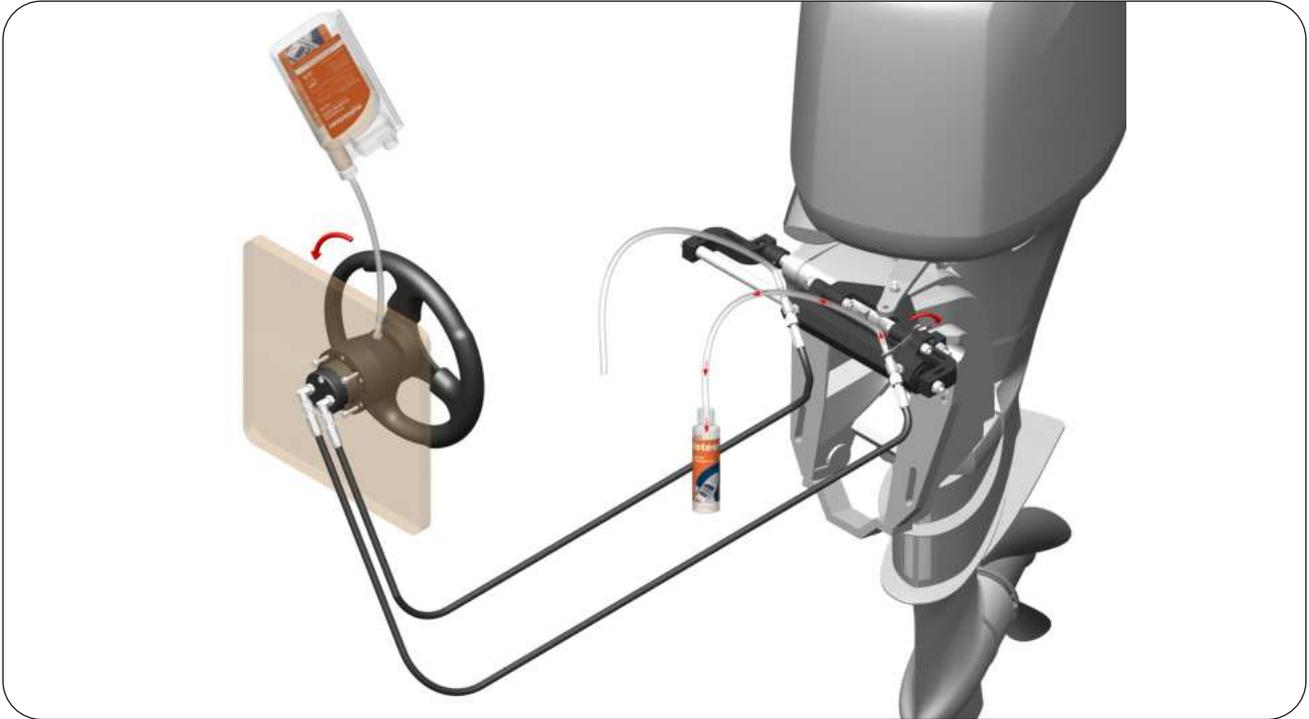
**STEP 14 :** Continue to turn the Steering Wheel towards Starboard Side. When the Oil comes out from air bleeder without air bubbles then carefully close the air bleeder. Do not overtighten the air bleeder. Continue to turn the Steering Wheel in the same direction to fill the Cylinder chamber. During this phase, the Cylinder body will move to the opposite direction up to the end stroke.
