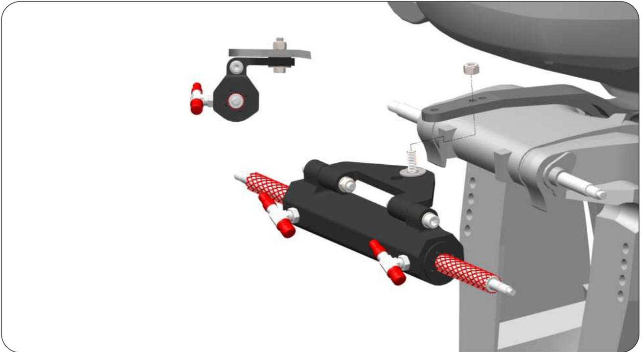
**STEP 6:** Remove the Piston Rod Protector before assembling the Support Bracket (4).
