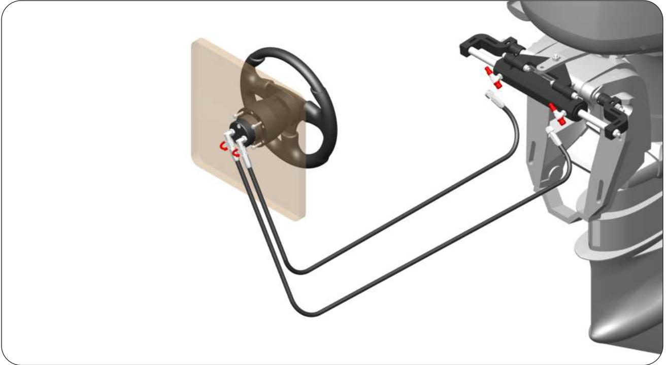
**STEP 4:** Remove the thread protector caps from both the T-Fitting Hose Side Port of Cylinder.
