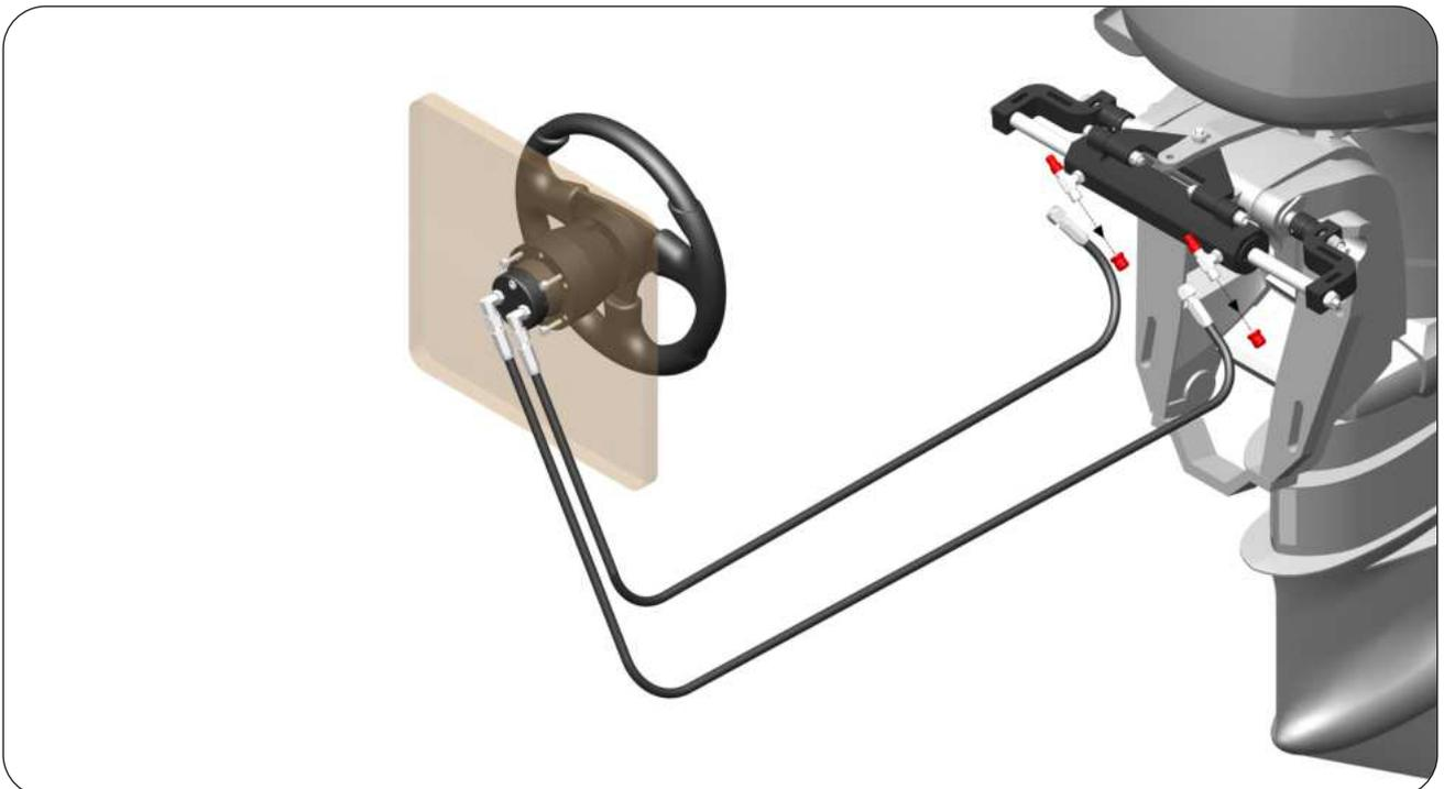
**STEP 5 :** Insert the Hose Fitting from Starboard Side of Helm into the Port Side Hose Fitting of Cylinder & vice versa. Tighten the Hex Nut on the Hose Fitting by using 19 mm Wrench with a torque of 15 Nm (52 lb ft).
