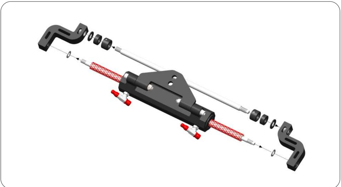
**STEP 3:** Apply Marine Grade Grease on the Center Shaft (3) and insert the Center Shaft into the Tilt Tube of Engine.
