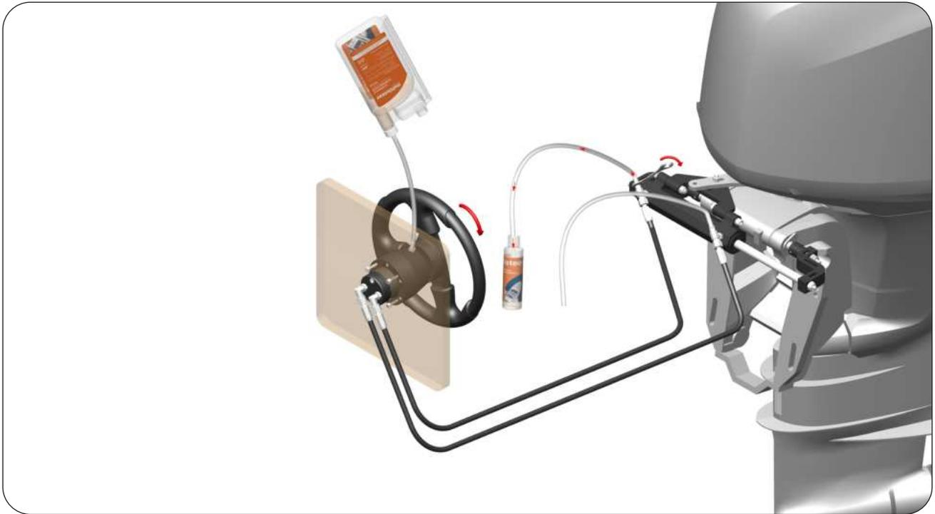
**STEP 16 :** Continue to turn the Steering Wheel towards Port Side. When the Oil comes out from air bleeder without air bubbles then carefully close the air bleeder. Do not overtight more than 15 Nm the air bleeder. Continue to turn the Steering Wheel in the same direction to fill the Cylinder chamber. During this phase the Cylinder body will move to the opposite direction up to the end stroke.
