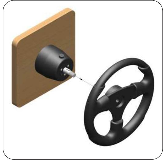
**STEP 2:** Apply grease lightly on the Tapered Shaft of the Helm. Slide the Steering Wheel supplied separately on the Helm Shaft.
