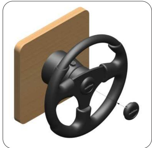
**STEP 4:** Fix the Wheel cap in the center of the Wheel where cap slot is provided.
