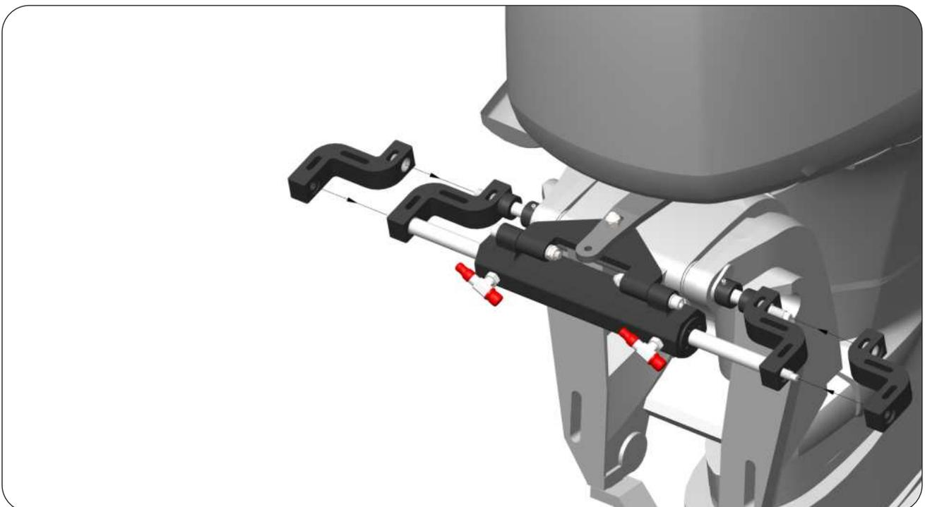
**STEP 9 :** Insert the Washers (10) and Nyloc Nut (11 & 12) on the two ends of the Support Rod (3) & Piston Rod (1) respectively. Grease the Nyloc Nut threads with any Anti-Seize Grease. Tighten first the Center Shaft Nuts and then Piston Rod Nut by using a 19 mm Wrench with a torque of 70 Nm (52 lb ft).
