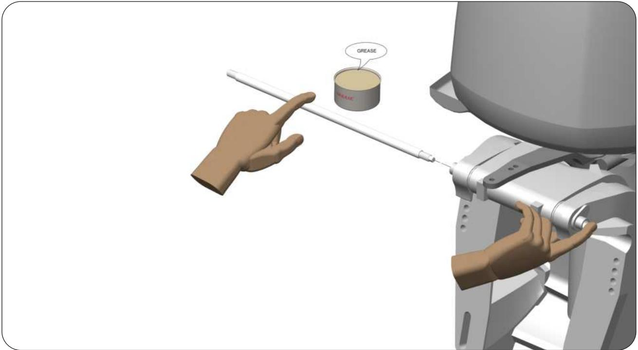
**STEP 4:** Assemble the Tiller Hex Stud Assembly (5) into the Tiller Plate (2) of Cylinder as shown.
